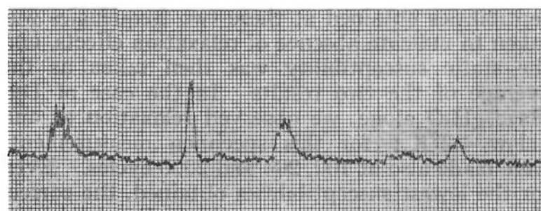
Fig. 1.—N.m.r. spectrum of 7-norbornadienyl fluoroborate in sulfur dioxide at -10^\circ . Peak positions are given in p.p.m. relative to tetramethylsilane as 10.00.
